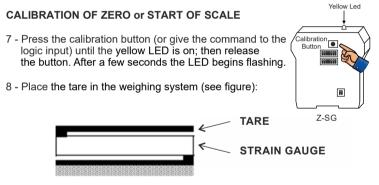
9 - Press the calibration button again (or give the command via the digital input) until the yellow LED turns off.
