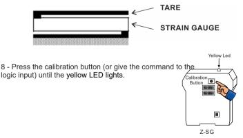
At this point the module has acquired the tare which will be used until the next calibration procedure.
