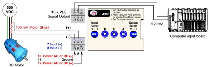
The API 4380 DIN switches are set to input select "V", Output select "I" and A=5, B=9, and C=3 for 100 mV input and 4-20 mA output. The API 4380 DIN powers the output loop, thus eliminating the need for an additional power supply. The 2000 V<sub>RMS</sub> 3-way isolation of the module protects against unexpected common mode voltages, ground loops and electrical noise.
