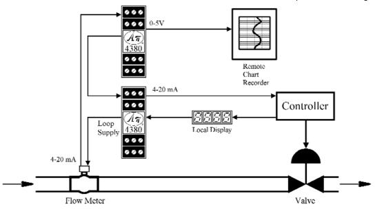
The flow meter is connected to a pair of API 4380 DIN Isolated, Field Ranging DC to DC Isolators. The first API 4380 DIN provides loop power for the flow meter from its built-in loop excitation supply, and its 4-20 mADC output drives both the local display and the flow controller. The second API 4380 DIN converts the 4-20 mADC signal from the flow meter to a 0-5 VDC signal which is sent to the remotely located chart recorder.
