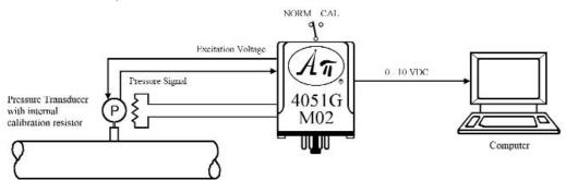
The API 4051 G M02 utilizes the pressure transducer's internal calibration resistor to unbalance the bridge to a specified value when the test switch is in the CAL position, ensuring accurate system calibration.
