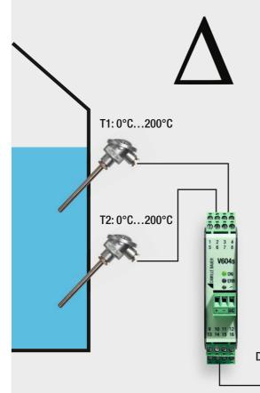
SINEAX V604s is predestined to monitor the difference of 2 input values as it is often the case in temperature monitoring.
