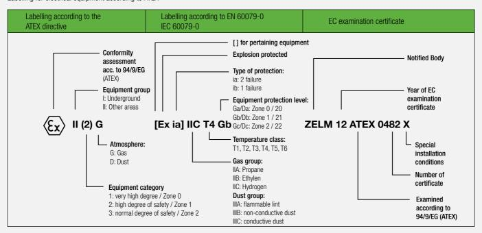
Labelling for electrical equipment according to IECEx
