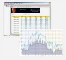
The .NET-based software facilitates the data acquisition and analysis of the optional data loggers and lists of SINEAX CAM and APLUS. The data will be stored in a database so that a much longer history is built up than would be the case if only the present memory content of the device was analysed. The program is capable of processing several devices simultaneously.
