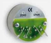
Wiring print with AMP connections
