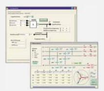
This software perwiths ONLINE/OFFLINE parawitherising of SINEAX CAM and APLUS as well as visualising measured values. It also supports users in commissioning and service. The program design is systemoriented and thus enables the simultaneous communication with several devices.
