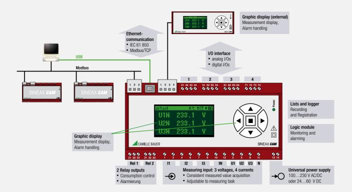
The optional 7-language graphic display (internal, external or both) is provided to visualise measured data and list entries on site. Users can adapt the display of measured data almost freely to their requirements. If required, a preferred display or
