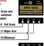
Cu 60/75°C 13 Power AC or DC + conductors 14 **Earth Ground** 14 AWG
