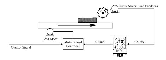
Conversely, decreasing load on the cutter increases the speed of the feed motor. The feed rate is controlled to maintain the optimum load on the cutter at all times. In addition, the 2000 VRMS isolation protects against unwanted ground loops and electrical noise commonly found in industrial environments.
